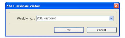
**Step 5** After the keyboard window is added, when creating Numerical Input and ASCII Input objects, "200. Keyboard" can be found in **[Data Entry]** » **[Keyboard]** »
