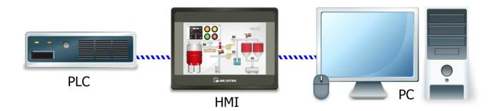
Pass-through provides two modes: [Ethernet] and [COM port].
