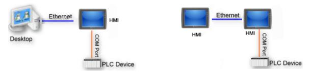
"Remote PLC" is a PLC being connected to a remote HMI. To control a remote PLC, add this type of device first. Please click [System Parameter Settings] » [New] to open [Device Properties] dialog. For example, use SIEMENS S7-200 as the Remote PLC:
