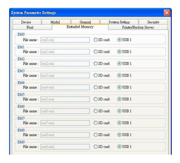
Extended Memory is numbered from EM0 to EM9. It works in a way similar to other device types (i.e. LW or RW address). Users can simply select from **[Device type]** list while adding a new object. Size of each extended memory is up to 2G word.
