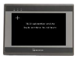
1. A "+" sign appears on the screen, touch the center of the sign, after all 5 signs are touched, "+" disappears and the touch screen parameters will be stored in HMI system.
